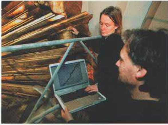
Fig. 5: Measuring crack width in stucco using microscope. Photo: H. Ekestang
